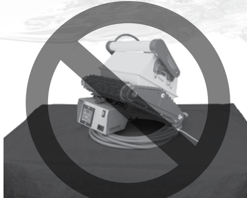
Incorrect (do not place cleaner on top of power supply)
